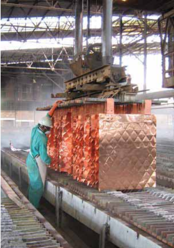
Worker with processed copper starter sheets at the Lulu Metallurgical Plant, which has a potential capacity of 175,000 tonnes of copper and 8,000 tonnes of cobalt per year
